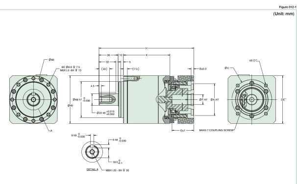
(Note) The dimension tolerances that are not specified vary depending on the manufacturing method. Please check the confirmation drawing or contact us for dimension tolerances not shown on the drawing above. Output shaft configuration shown is J6 (with a key and center tapped hole). J8 configuration has no key.
