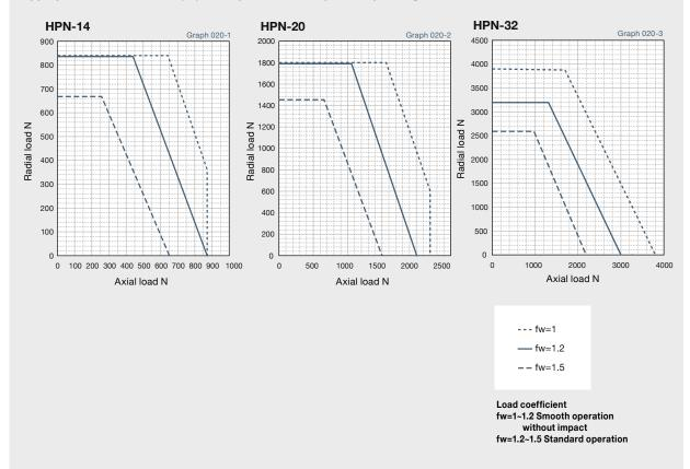
Output shaft speed - 100 rpm, bearing life is based on 20,000 hours. The load-point is based on shaft center of radial load and axial load.
