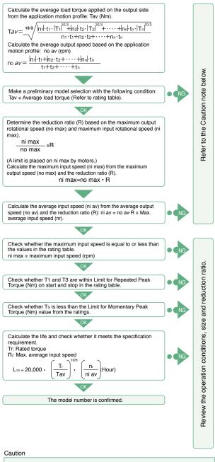
If any of the following conditions exist, please consider selecting the next larger speed reducer, reduce the operating loads or reduce the operating speed. If this cannot be done, please contact Harmonic Drive LLC. Exercise caution especially when the duty cycle is close to continuous operation.
